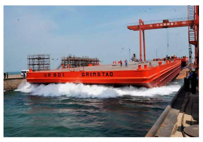
Built at Changxing Dalian Shipyard in China, the 9 019-deadweight tonne flat top barges were successfully launched on 7 June 2013.
